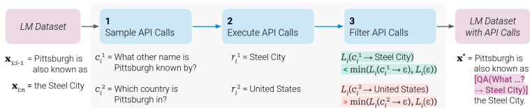
Figure 2: Key steps in our approach, illustrated for a question answering tool: Given an input text \mathbf{x} , we first sample a position i and corresponding API call candidates c_i^1, c_i^2, \dots, c_i^k . We then execute these API calls and filter out all calls which do not reduce the loss L_i over the next tokens. All remaining API calls are interleaved with the original text, resulting in a new text \mathbf{x}^* .
